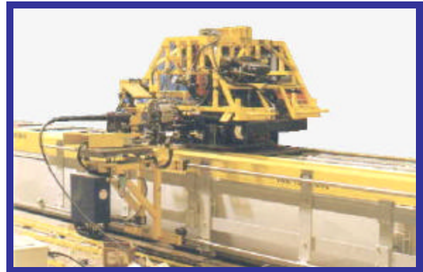
Zone & Continuous Running Sub-assembly Conveyor for Front Suspension & Engine Assembly
