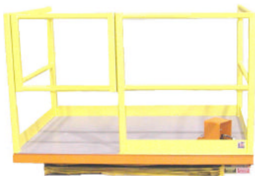
32" travel air / water lift with foot control, hand rails, access gate and toe plate.
